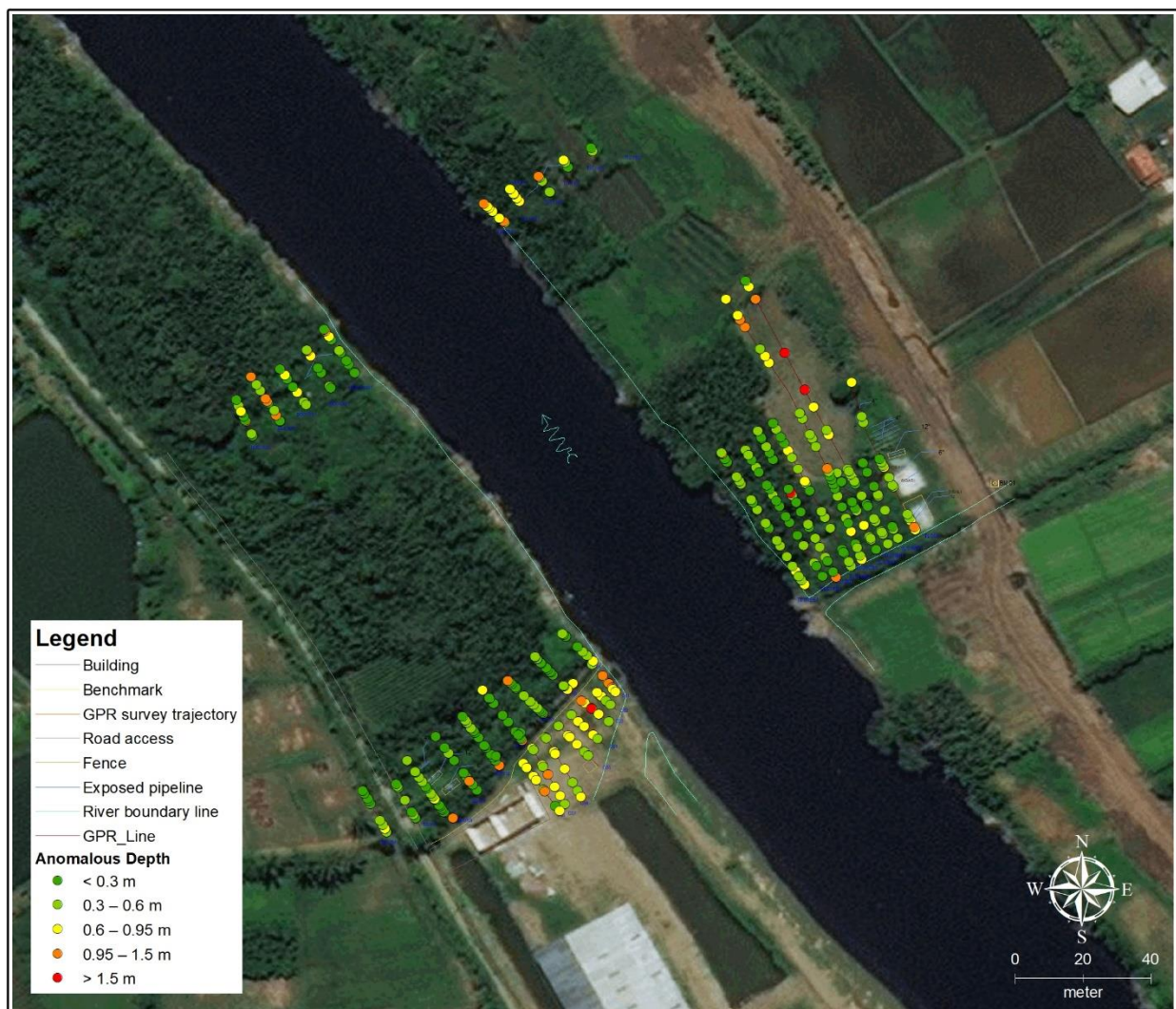
Figure 3 Lateral anomaly distribution of the object obtained from processed radargram.
